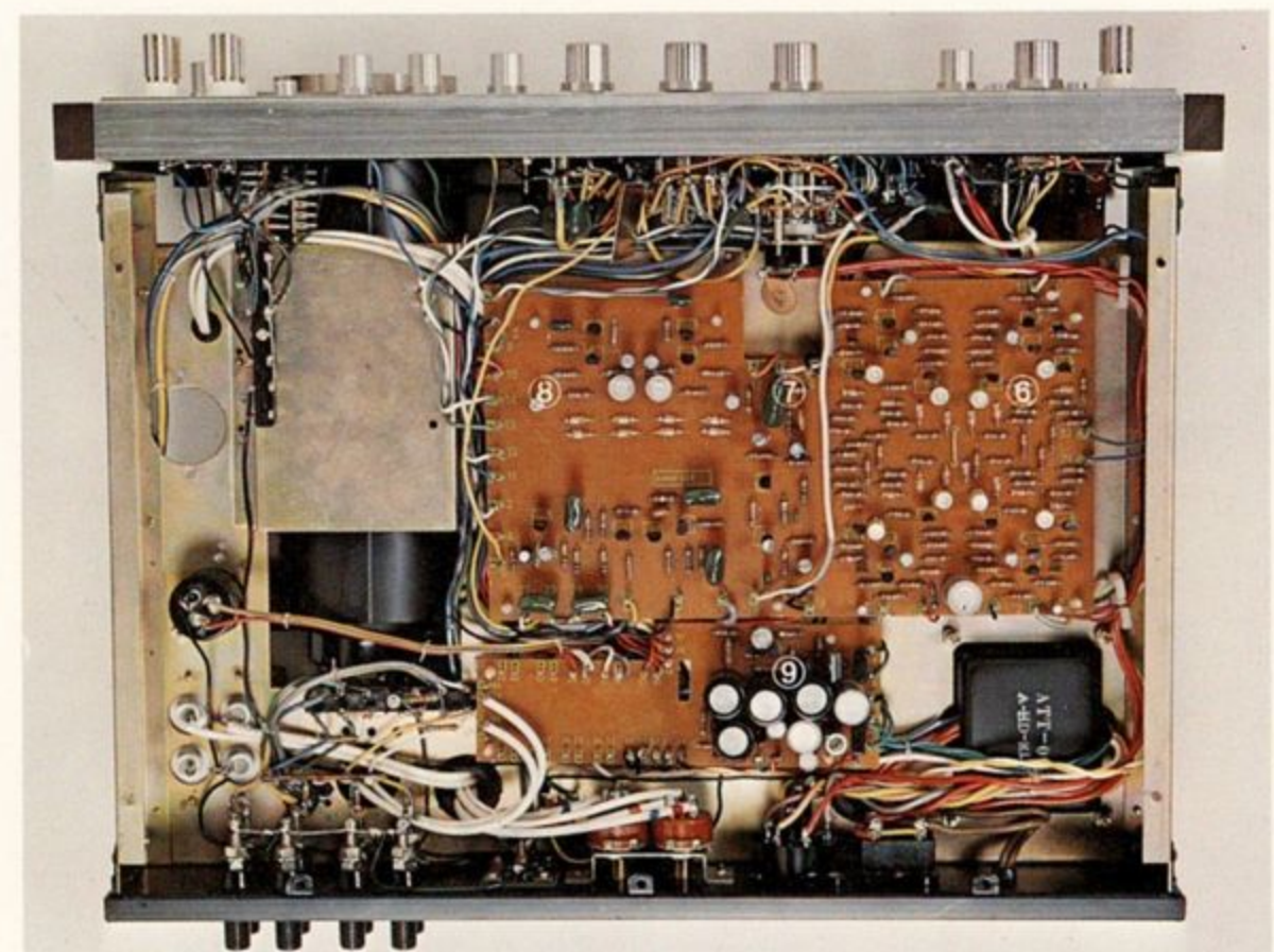
BOTTOM VIEW: ⑥ 4-CH. DISPLAY AMP. SECTION ⑦ MICROPHONE AMP. SECTION ⑧ METER AMP. SECTION ⑨ POWER SUPPLY UNIT
